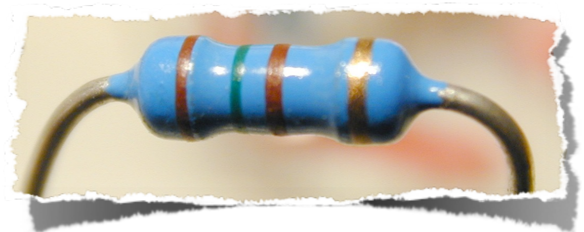
A 2500 \Omega resistor (each colour indicates one of the numbers)
