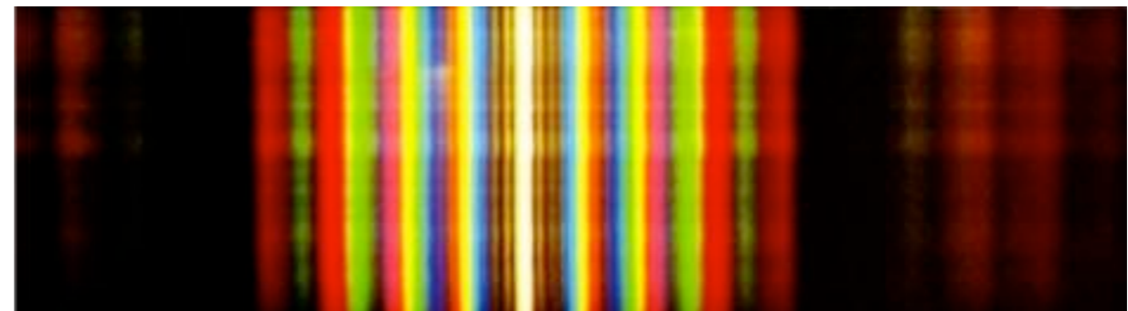
White light source: colour bands due to the increased / decreased intensity of particular wavelengths.
