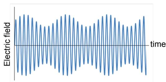
The signal is now being carried on the carrier wave. There is a need for the carrier wave to have a frequency much greater than the signal, otherwise it will do a poor job of representing the signal being sent. (A carrier wave can be any EM radiation).
