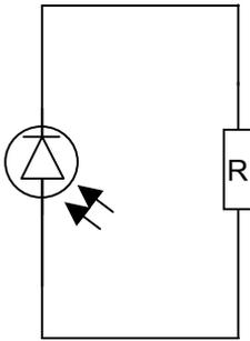
When a photodiode is *reverse biased*, very little current flows, but it is very sensitive to changes in light intensity.
