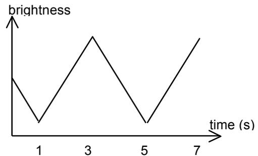
The brightness needs to be above zero, because the LED is always on.
