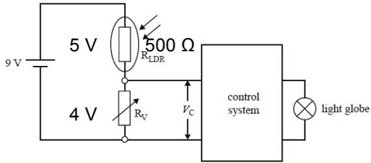
If the voltage across the control system needs to be 4 V for the light to turn on, then the voltage across the LDR is 5 V.
